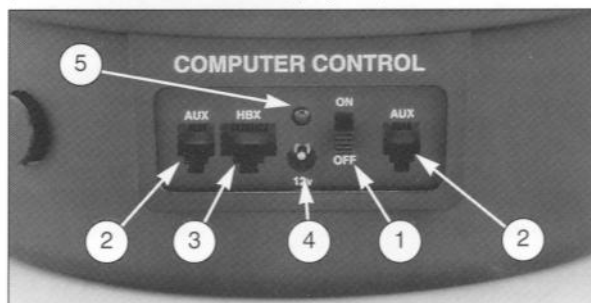
Fig. 4: Computer Control Panel. (1) ON/OFF Switch; (2) Auxiliary Ports; (3) Handbox Port; (4) 12v Connector; (5) Power Indicator Light.
